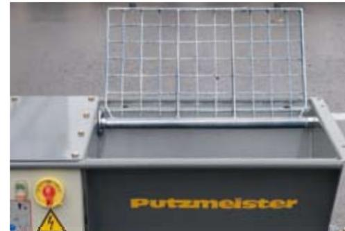
The safety grille can be opened extremely wide, so that it is easy to access the conveyor hopper (e.g. for cleaning).
