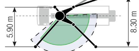
Support width based on center of support leg
